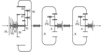
Figure 5. Kinematic scheme of the 3 planetary systems of the 7G Tronic automatic gearbox
