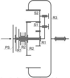
Figure 2. Kinematic scheme of a "Ravigneaux" planetary gear system
