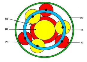
Figure 1. "Ravigneaux" planetary gear system
