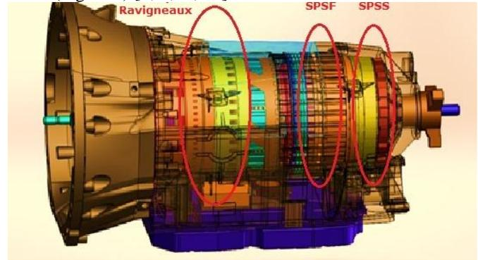
Figure 3. 7G Tronic automatic gearbox
