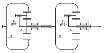
Figure 4 simple front planetary system SPSF and simple rear planetary system SPSS (A-central sun gear, B-crown gear, C<PS>carrier)
