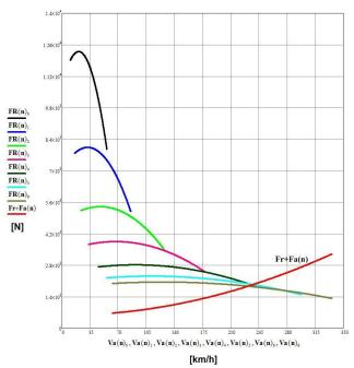
Figure 8. Traction and speed characteristics on all seven gears
