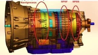
Figure 3. 7G Tronic automatic gearbox
