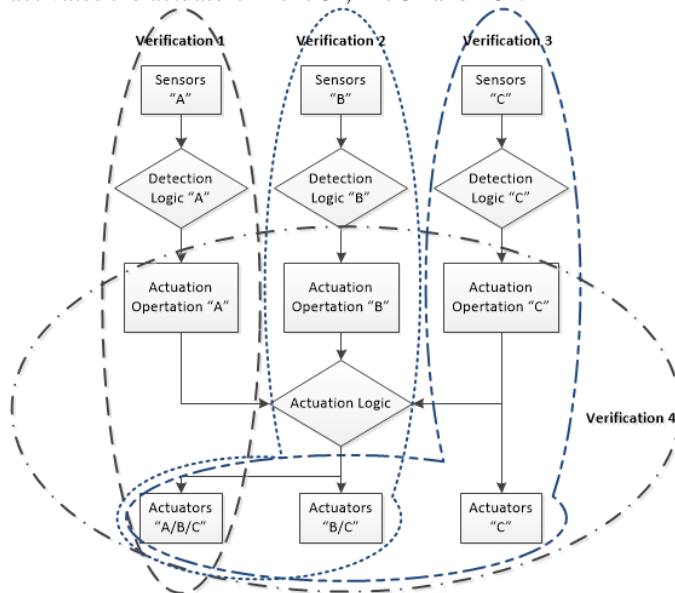
Fig. 4 - Mitigation program structure
