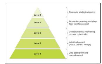
Fig. 1: Automation Pyramid Source: adapted of Webb and Greshock, 1990 [2]
