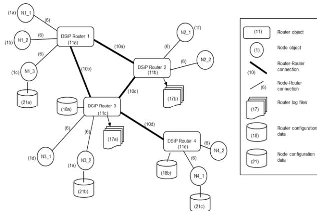
Fig. 5 Blueprint of DSiP network solution [10]
