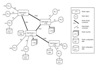
Fig. 5 Blueprint of DSiP network solution [10]
