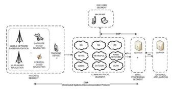
Fig. 4 Modular system-level description of improved tracking system for emergency response
