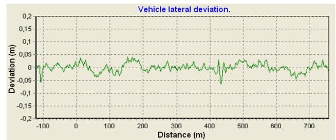
Fig. 11 (a) radius of curvature of the route segment between Mercado and Pedro II Stations in Expresso Tiradentes bus corridor (b) lateral deviation of vehicle along the same segmen
