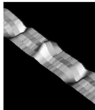
Fig. 6 3D view of the magnetic field profile generated by a track of magnets installed in the bus corridor
