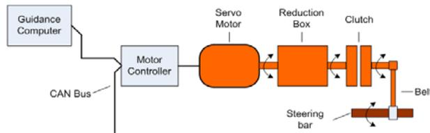
Fig. 9 functional block diagram of wheel steering actuator
