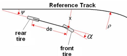
Fig. 7 vehicle dynamics of the BRT bus representation based on bicycle model.
