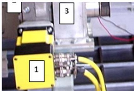
Fig. 10 assembly of wheel steering actuator. (1) servomotor; (2) reduction box; (3) magnetic clutch; (4) steering bar
