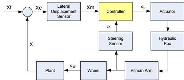
Fig. 8 functional block diagram of the magnetic guidance system
