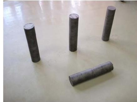
Fig. 5 pictures of magnetic markers (permanent magnet of ferrite, dimension: 25x100 mm)
