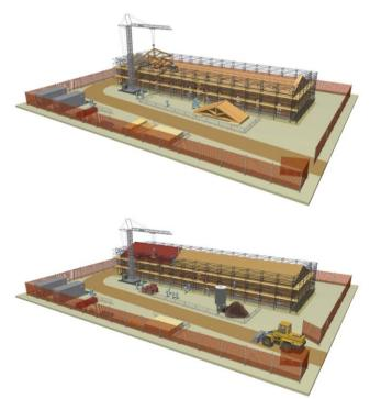
Fig. 5 (a, b), use the 3D model for worksite and planning. First phase: setting up of building site and surroundings, demolition, existing covering removal and new truss positioning. Second phase: conclusion of covering system installation, wall restoration, frameworks, inside works, plants and finishings, outside arrangements
