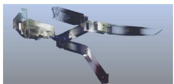
Fig. 3, survey point cloud of basement level, ex Arsenale Verona
