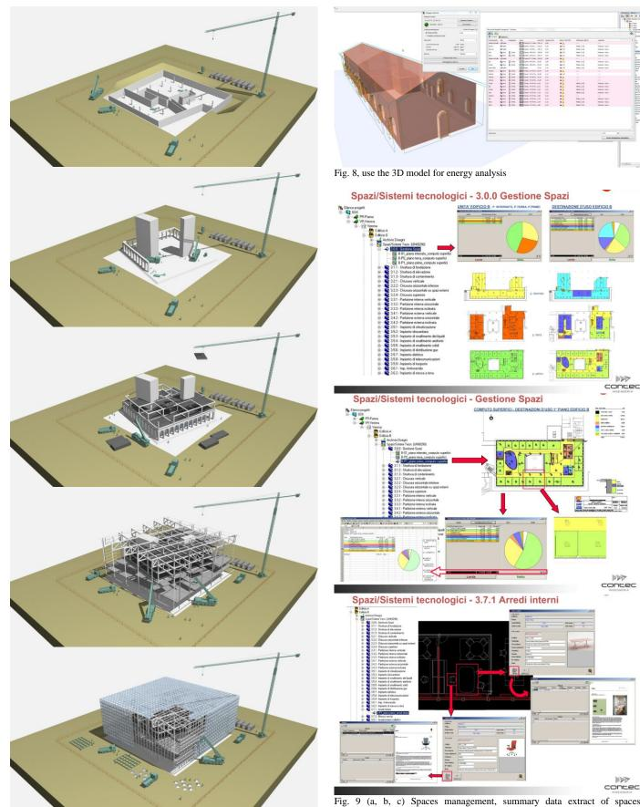
Fig. 7 (a, b, c, d, e) Building site, foundations and basements, structures of stiff units, prefabricate ground structures, covering steel structure, closeout structure
