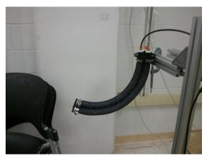
**Figure 6.** Section of new continuum robot demonstrating the constant curvature property.
