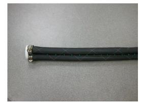
Figure 2. Three muscles connected by zip ties at regular intervals to form a section.
