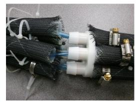
Figure 4. Internal air supply hose connections using manifolds.
