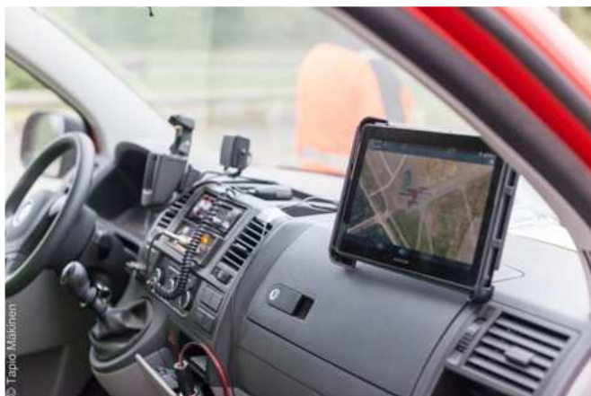
Fig. 4 Smartphone installation on fire truck. (Photo courtesy of Tapio Mäkinen.)
