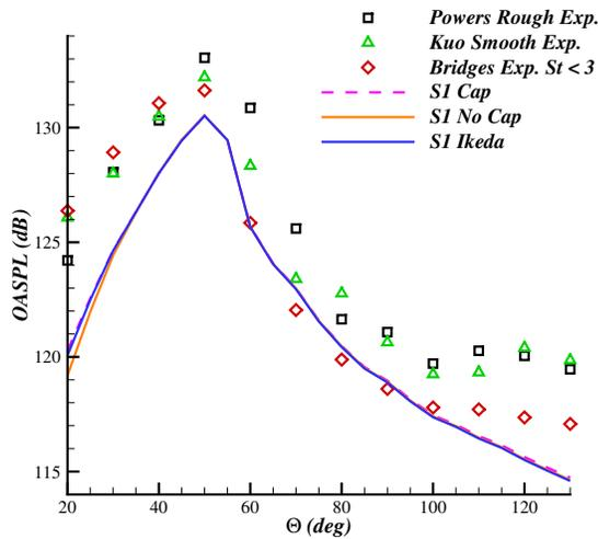
Fig. 4: Baseline nozzle OASPL results at  $r = 200R_j$  for FWH surface S1 and various end-cap treatments.
