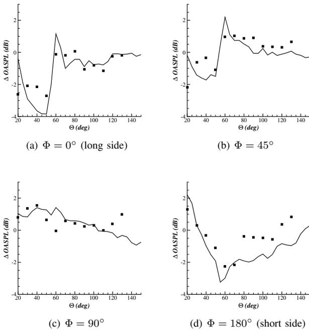
Fig. 5: Change in OASPL between baseline and  $35^\circ$  beveled nozzles using FWH surface S2 and the Ikeda et al. [74] end-cap method. Lines are used for the simulation data and the symbols are for the experiment.
