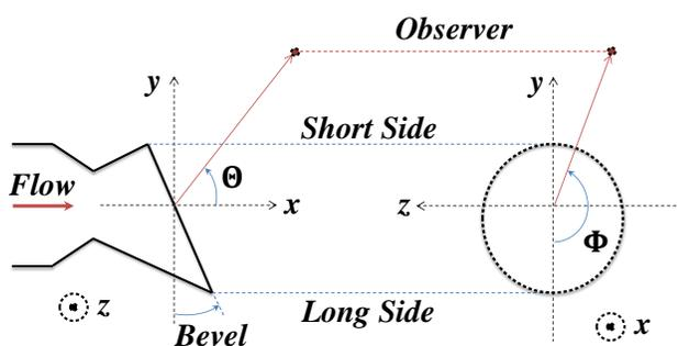
Fig. 1: Definition of the nozzle bevel angle, the long and short sides of the beveled nozzle, and the azimuthal angle,  $\Phi$ .
