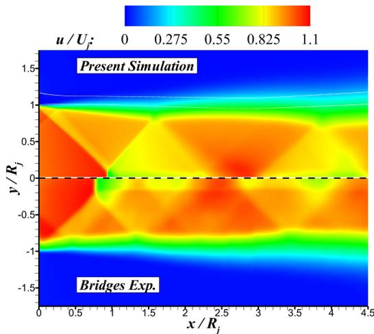
Fig. 2: Comparisons between mean simulation and particle image velocimetry (PIV) experimental data ( $u/U_j$ ) for the baseline jet.
