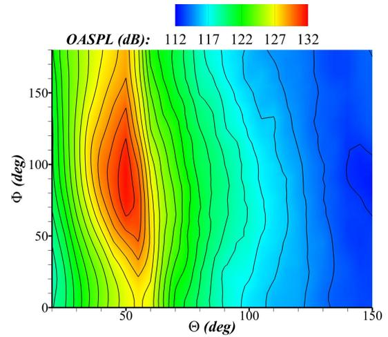
(a) OASPL at  $r = 200R_j$ . Contour lines are spaced every 1 dB.
