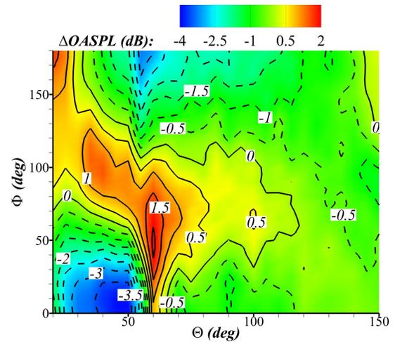
(b)  $\Delta OASPL$ . Contour lines are spaced every 0.5 dB and dashed lines negative.
