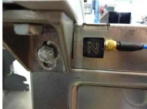
**Figure 12 – Accelerometer positioned near one bolt**
