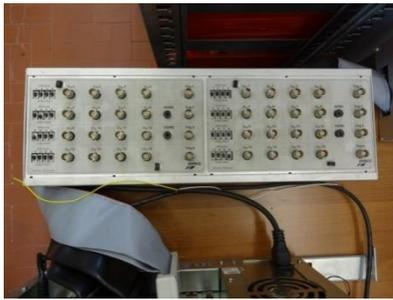
Figure 2: DSpace Control System A/D board
