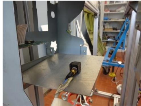
**Figure 13 – Accelerometer positioned on the clamped board**
