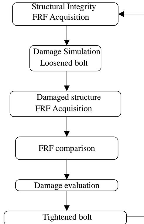
**Figure 8 - Hypothetic situation to test the SHM tool**
