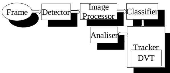
Fig.2 Components of a video surveillance system
