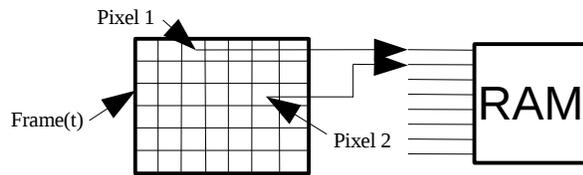
Fig. 8 if pixel 1 > pixel 2 than pixel 1 is quantized to 1. Pixel 1 is quantized to 0 otherwise.
