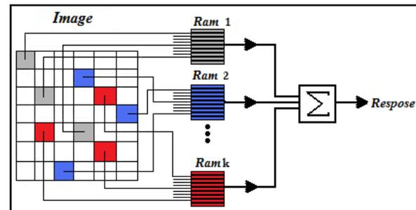
Fig. 3 WiSARD discriminator: a discriminator with  $k$  RAMs of 9bit bus address where every bit is connected to a quantized pixel. Being represented only three of nine pixels connected to each RAM.
