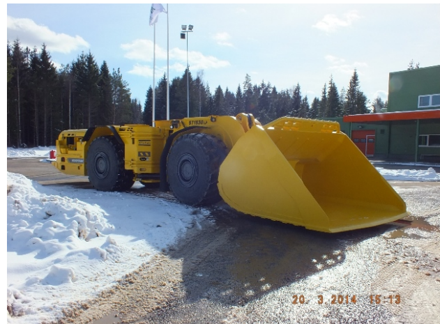
Fig. 1. Underground loader. Picture by courtesy of VKG AS.
