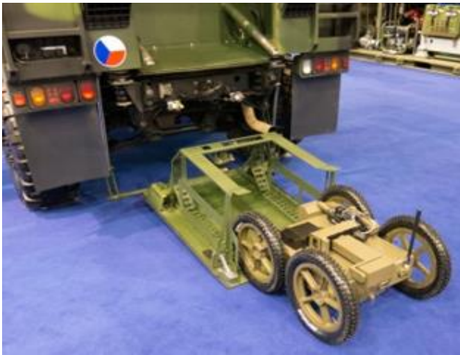
Fig. 2 Orpheus-AC2 military robot for CBRN operator-controlled reconnaissance, robot-retaining system detail
