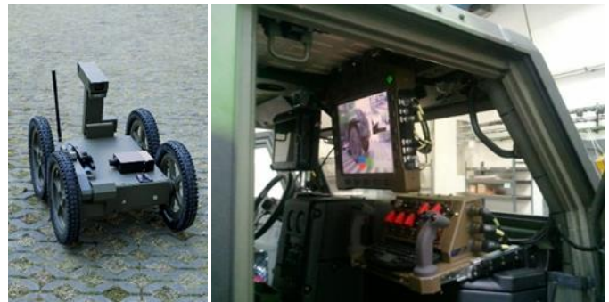
Fig. 1 Orpheus-AC2 military robot for CBRN operator-controlled reconnaissance – the robot (left), operator's station inside the armored car (right)
