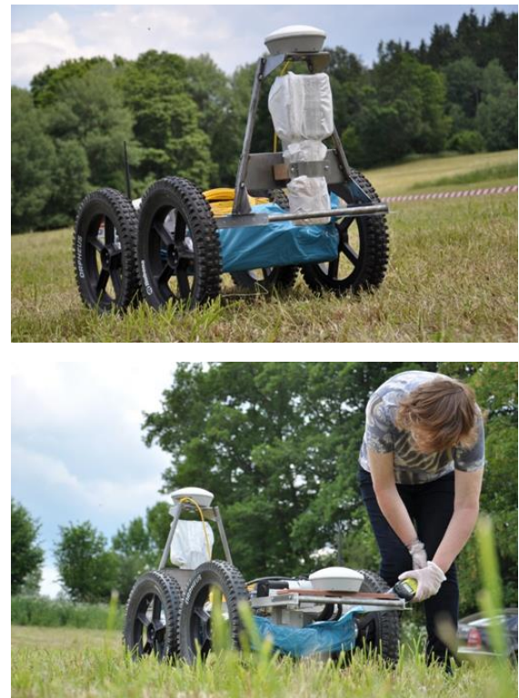
Fig. 5 Orpheus robot during the first experiment. Vital parts were covered by plastic bags as radiation dust protection (up); the robot has to be measured and eventually decontaminated (down).
