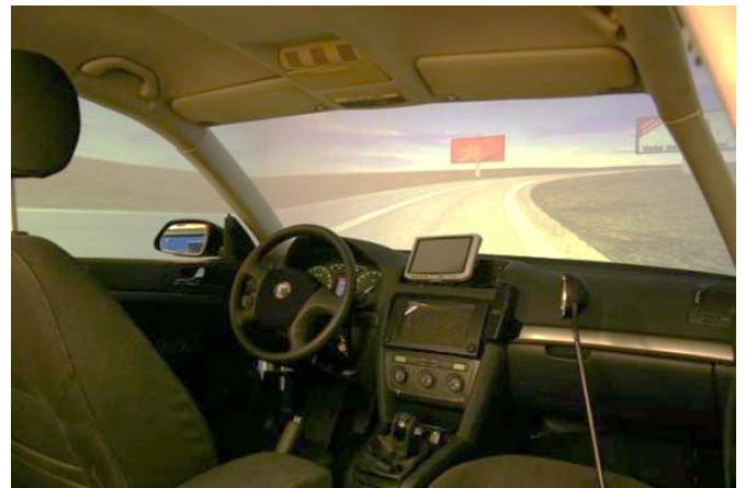
Fig. 13: Cockpit of the light simulator Octavia II 3D (2010) equipped with 3DOF moving platform, specially designed for use with light simulator
