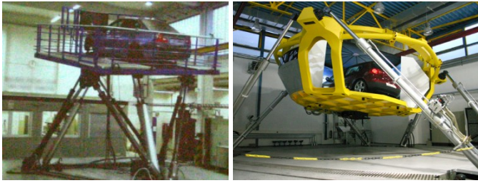
Fig. 5: Full car simulator situated on robust hexapod platform in BMW – left and one of the European latest simulators in DLR – right
