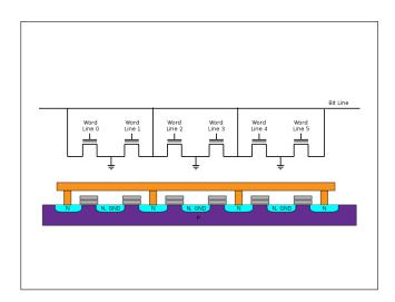
Fig. 1 Wiring of NOR flash memory [6]
