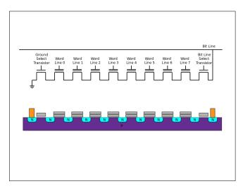
Fig. 2 Wiring of NAND flash memory [6]
