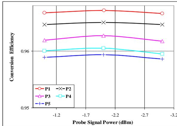
Fig. 6 Variation of probing signal ( $P_0$ ) versus conversion efficiency at  $P_1=0$ ,  $P_2=2$ ,  $P_3=2.5$ ,  $P_4=3$  and  $P_5=3$  dBm and  $I=250$  mA
