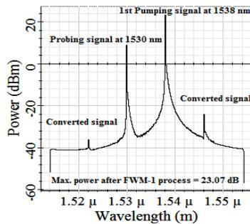
Fig. 11 Converted signals after exposing two signals (combining signals) to TW-SOA-1
