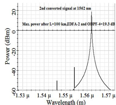
Fig. 19 2<sup>nd</sup> converted signal after spanning 100 km, then exposing to EDFA-2 and OBPF-4
