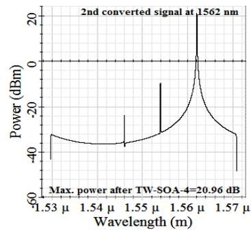
Fig. 17 2<sup>nd</sup> converted signal after applying DEMUX-2 and TW-SOA-4
