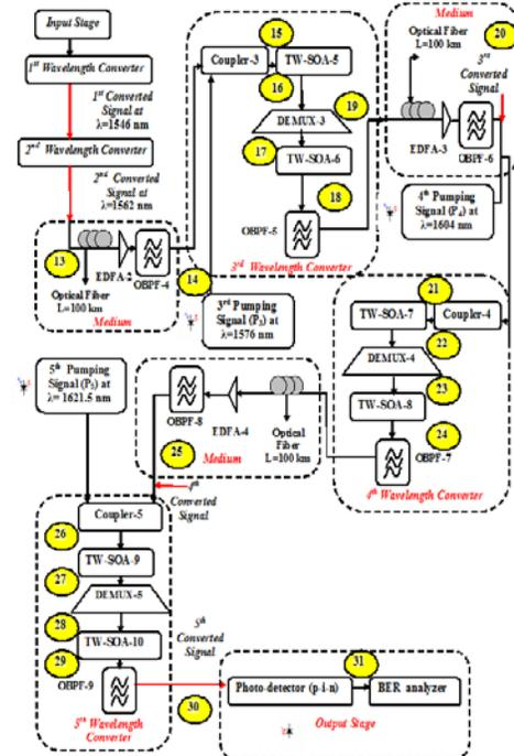
Fig. 4 Proposed setup for five-cascaded wavelength conversion spanning 400 km transmission
