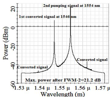
Fig. 16 2<sup>nd</sup> pumping and 1<sup>st</sup> converted signals coupled using 3-dB-coupler-2 and introduced to TW-SOA-3
