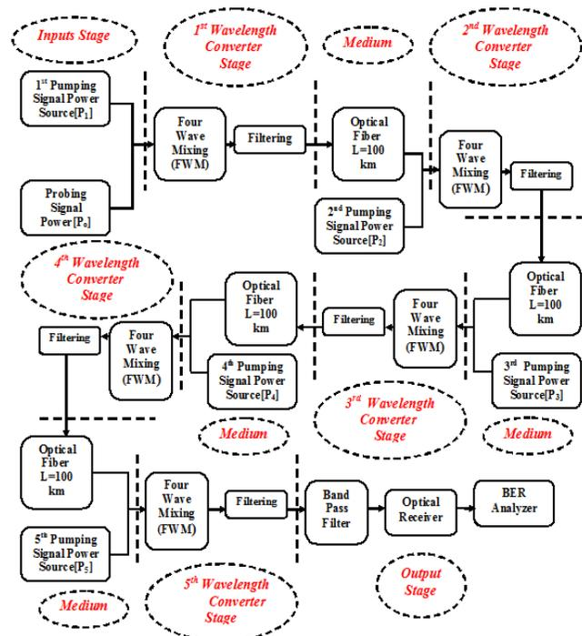
Fig. 2 General block diagram for the five-cascaded stages SOA-based wavelength converter
