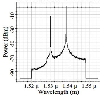
Fig. 10 1<sup>st</sup> pumping and probing signals combined together using a 3-dB coupler-1
