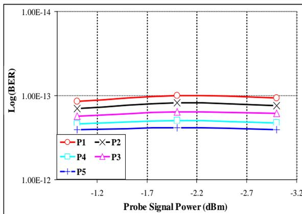
Fig. 7 Variation of probing signal ( $P_0$ ) versus BER at  $P_1=0$ ,  $P_2=2$ ,  $P_3=2.5$ ,  $P_4=3$  and  $P_5=3$  dBm and  $I=250$  mA
