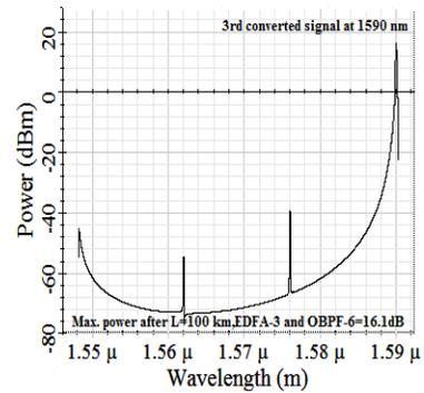
Fig. 22 3<sup>rd</sup> converted signal after spanning 100 Km, then exposing to EDFA-3 and OBPF-6
