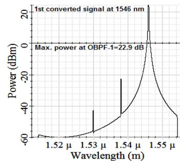
Fig. 13 1<sup>st</sup> converted signal after exposing to OBPF-1
