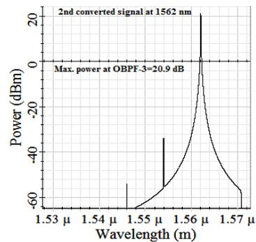
Fig. 18 2<sup>nd</sup> converted signal after Exposing to OBPF-3
