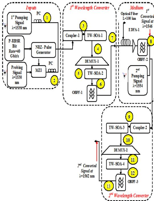
Fig. 3 Proposed setup for two-cascaded wavelength conversion spanning 100 km transmission in a single-mode fiber. PC: Polarization Controller, EDFA: Erbium-Doped Fiber Amplifier, OBPF: Optical Band-Pass Filter, MZI: MOD: LiNbO3 Mach-Zehnder Modulator, TW-SOA: Traveling Wave Semiconductor Optical Amplifier, P-RBSR: Pseudo-Random Bit Signal Generator, NRZ: Non-Return to Zero, DEMUX: Demultiplexer.
