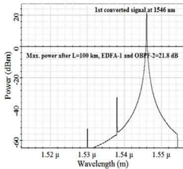
Fig. 14 1<sup>st</sup> converted signal after spanning 100 km, Then exposing to EDFA-1 and OBPF-2
