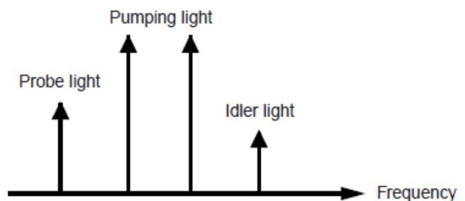
Fig. 1 Schematic of four-wave mixing in the frequency domain for two-channel pump wave
