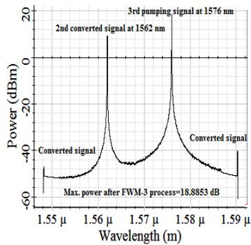
Fig. 21 3<sup>rd</sup> converted signal after applying DEMUX-3, TW-SOA-6 and OBPF-5
