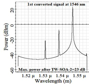
Fig. 12 1<sup>st</sup> converted signal after applying DEMUX-1 and TW-SOA-2
