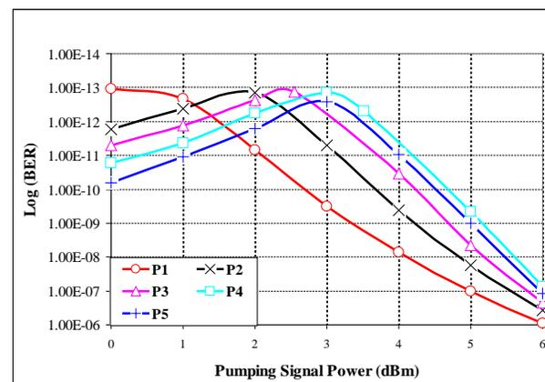
Fig. 5 Variation of pumping signals versus BER at P<sub>0</sub> = -2 dBm and I = 250 mA
