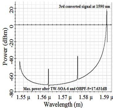
Fig. 20 3<sup>rd</sup> pumping and 2<sup>nd</sup> converted signals coupled using 3-dB-coupler-3 and introduced to TW-SOA-5
