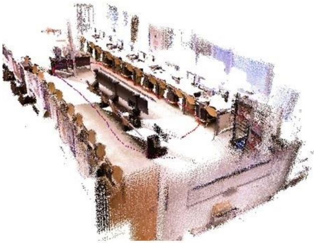
Fig. 6. Result of the algorithm on own datasets. This dataset includes 310 image pair. The image shows three dimensional and two dimensional maps from one laboratory of the university.
