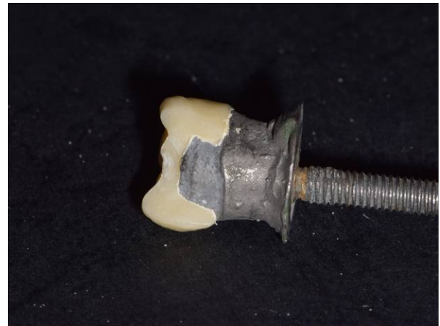
Fig. 9. Fracture of the crown after cyclic loading (800 N).
