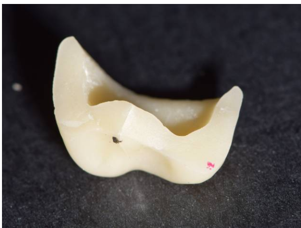
Fig. 8. Section view after cyclic loading.
