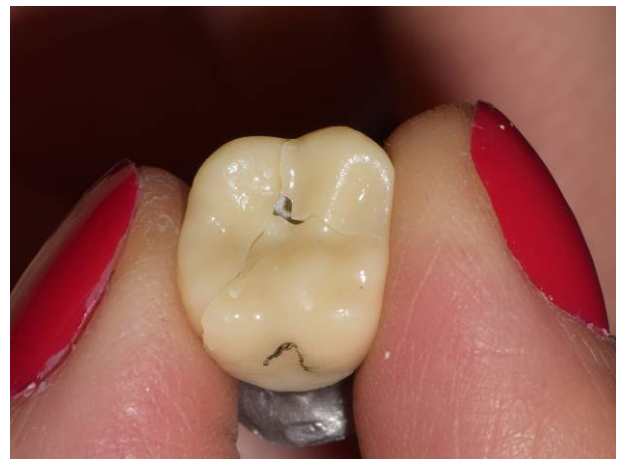
Fig. 4. Fracture lines and in the crowns initiated from the loading point, after static loading (1200 N).
