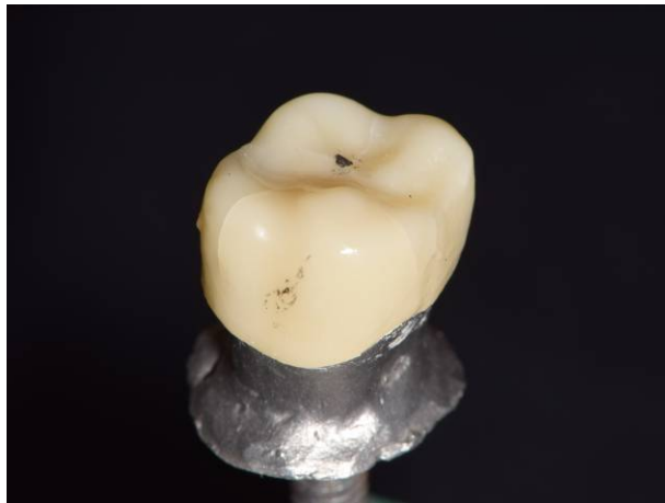
Fig. 6. Cracks in the crown after cyclic loading (550 N).
