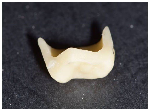
Fig. 5. Section view of one fragment after static loading.
