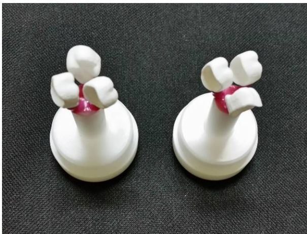
Fig. 2. Wax pattern of the crowns prepared for investing.
