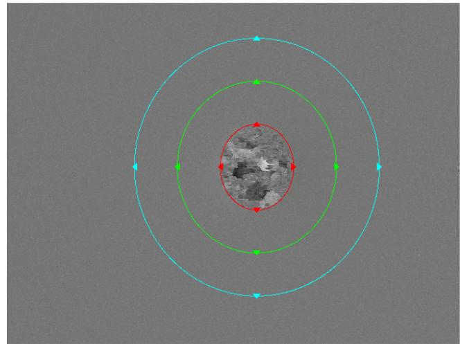
**Fig. 8** Calculated phase map for a hole drilled at 5000 rpm
