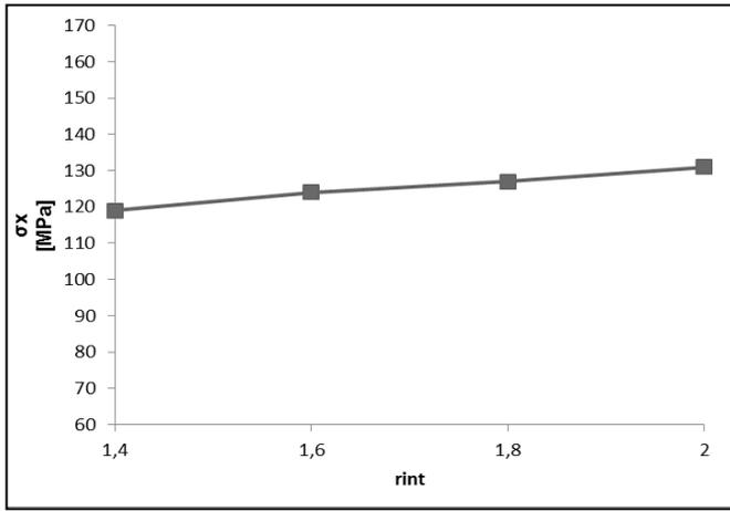
**Fig. 6** Calculated  $\sigma_x$  stress as a function of the internal radius of analysis. Drilling rotation speed: 5.000 rpm
