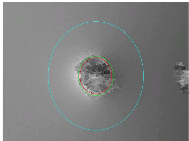
**Fig. 10** Calculated phase map for a hole drilled at 50000 rpm
