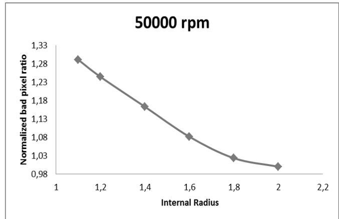
**Fig. 9** Bad pixel ratio as a function of the internal radius of analysis. Drilling rotation speed: 50000 rpm.
