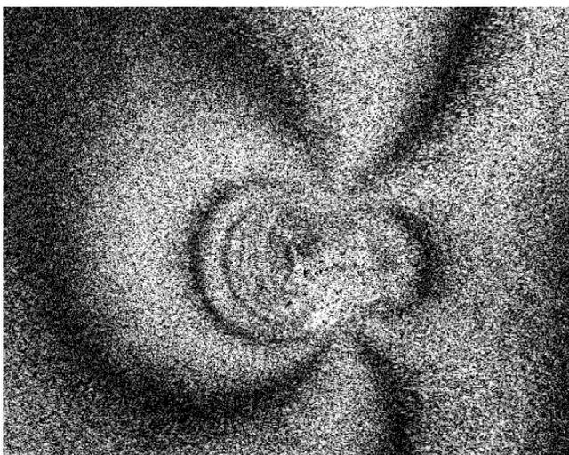
**Fig. 3** Exemplary fringe pattern recorded during the drilling process. Fringes represents the lines of iso-displacement with respect to the direction of sensitivity of the interferometric system
