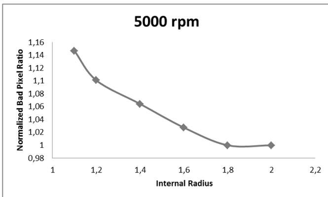
**Fig. 7** Bad pixel ratio as a function of the internal radius of analysis. Drilling rotation speed: 5000 rpm..
