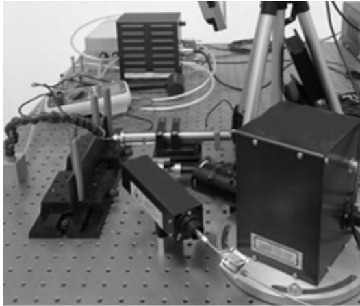
**Fig. 2** Experimental set-up adopted for HDM-ESPI evaluation of RS
