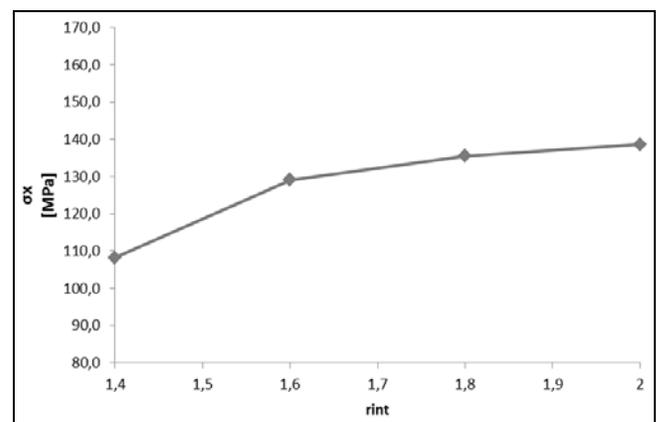
**Fig. 5** Calculated  $\sigma_x$  stress as a function of the internal radius of analysis. Drilling Rotation speed: 50000 rpm
