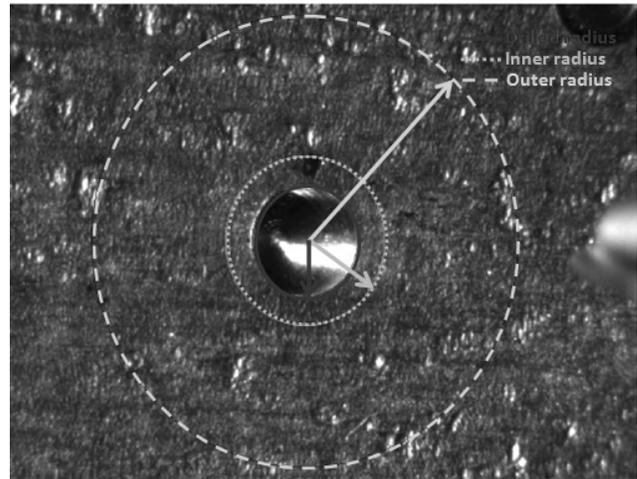
**Fig. 4** Screenshot of the area of analysis included between the outer circle (dashed line) and the inner circle (dotted line). The solid line identifies the drilled hole.
