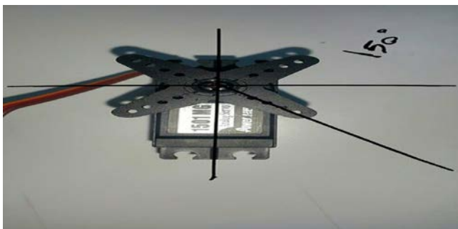
Fig.5: Servo motor with angle 150 degrees.
