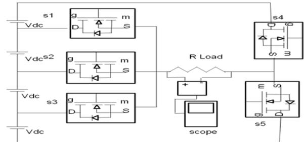
Fig. 7 Proposed Power circuit for 7-level output .
