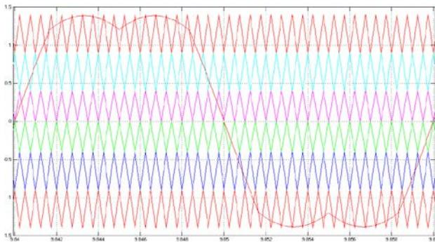
Fig 6: switching sequence of svpwm for single space.
