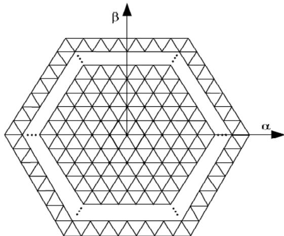
Fig 2. State vectors space for N-level cascaded multilevel inverter
