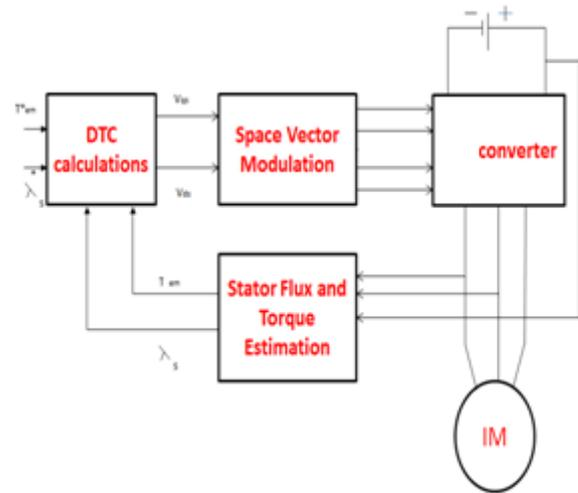
Fig 1. DTC using space vector modulation block diagram
