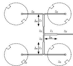
Fig. 2 Routing wire pattern for parallel array arrangement of the array antenna in Fig. 1.
