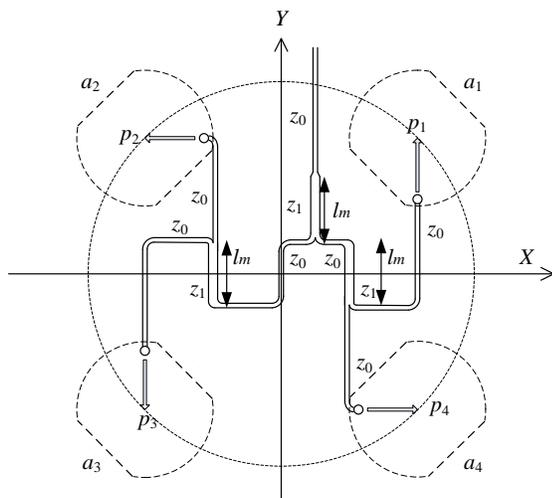
Fig. 10 Routing wires for the orthogonal array antenna (arrangement 1).
