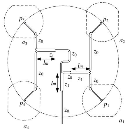
Fig. 12 Routing wires for the orthogonal array antenna (arrangement 2).
