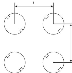
Fig. 1 An example of circular polarized plane antenna array by Haneishi, et al [2].
