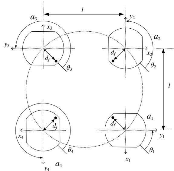
Fig. 11 An array antenna with orthogonal arrangement (arrangement 2).
