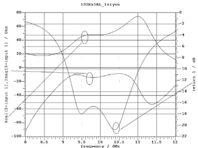
Fig. 6 Return loss and input impedance.
