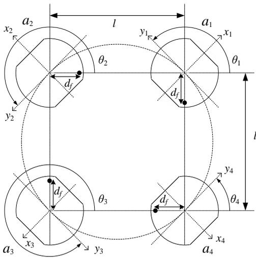
Fig. 9 An array antenna with orthogonal arrangement (arrangement 1).
