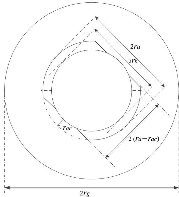
Fig. 3 Overhead view of a unit circular polarization antenna with three elements.
