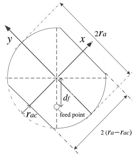
Fig. 4 Dimension of feeding element.
