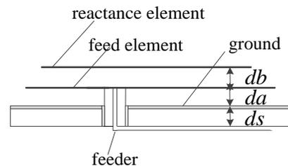
Fig. 5 Cross-sectional view of the unit circular polarization antenna with three elements and a feeding circuit.
