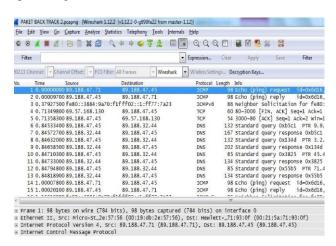
Figure 4. Intercepted packets from all IP addresses in the network, without the use of filters
