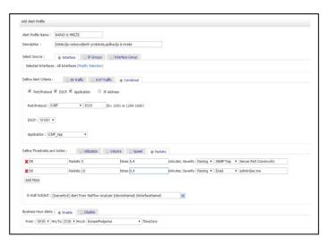
Fig. 11. Sending SNMP Trap alert messages for the ICMP protocol, DSCP-101001 and ICMP application  $\,$
