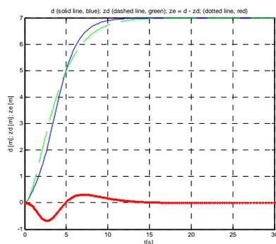
Fig. 3. Time history of the trolley displacement (blue solid line), desired trajectory (green dashed line), and tracking error (red dotted line)
