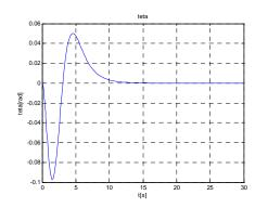
Fig. 2. Time history of the swing angle of the payload
