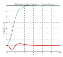
Fig. 3. Time history of the trolley displacement (blue solid line), desired trajectory (green dashed line), and tracking error (red dotted line)
