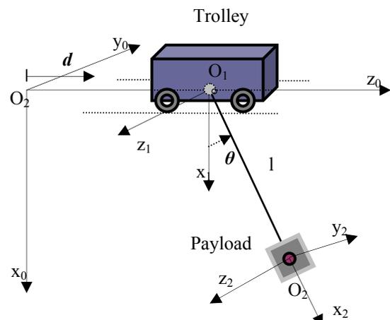
Fig. 1. Schematic of the overhead crane
