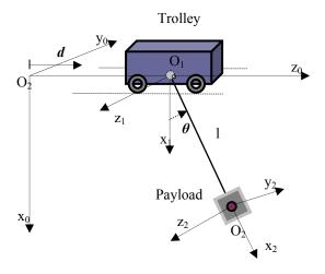
Fig. 1. Schematic of the overhead crane
