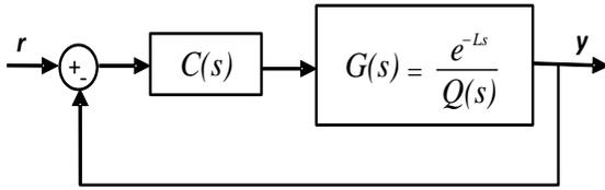
Fig. 1 Classical feedback system where the system's transfer function is given by
