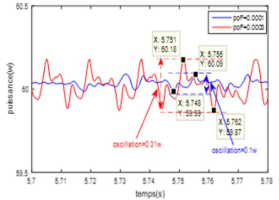
Fig 17 Fixed step: Oscillation around MPP.
