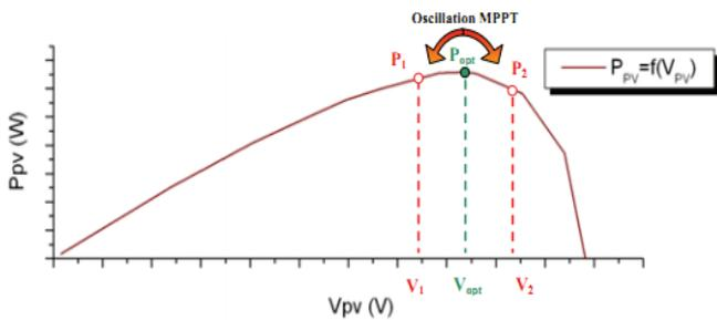
Fig. 6 Oscillation around the MPP [10].
