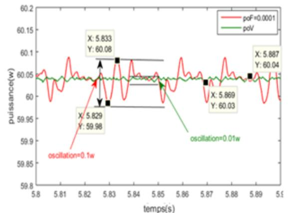
Fig 20 Variable step: Oscillation around MPP.
