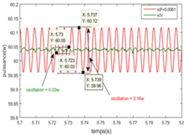
Fig 14 Variable step: Oscillation around MPP.
