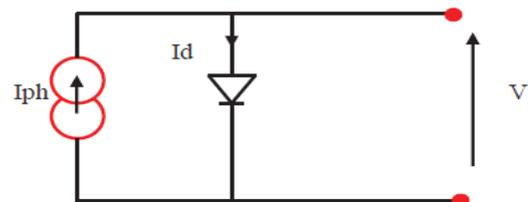
Fig.1 Ideal model of PV cell [6].
