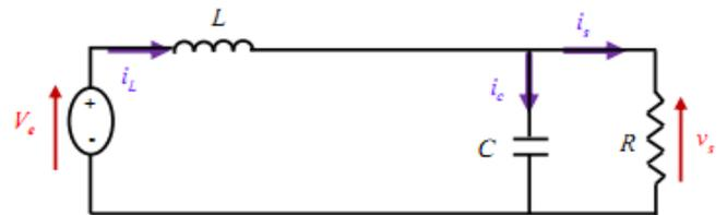
Fig. 5. Circuit equivalent when switch K is open [4].
