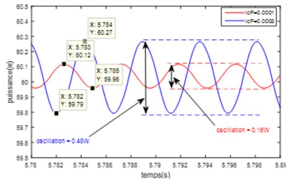
Fig 11 Fixed step: Oscillation around MPP.
