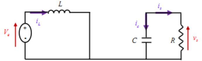
Fig. 4 Circuit equivalent when switch K is closed [4].
