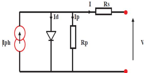
Fig.2 Single Diode Model of PV cell [6].
