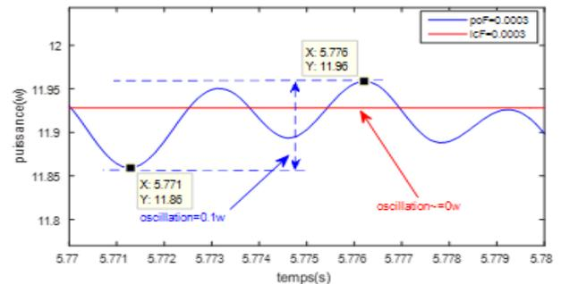
Fig. 25 Comparison results: Oscillation at 200W/m<sup>2</sup>.
