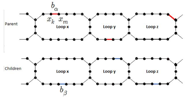
**Fig. 4.** Mutation in three independent loops (----- open arc in children chromosome, ----- open arc in parent chromosome)
