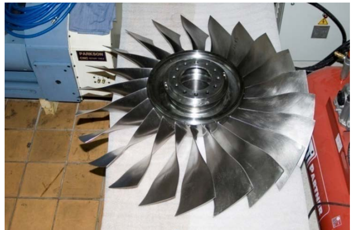
Fig.2. Fan blisk manufactured by COMOTI during SILENCE-R project
