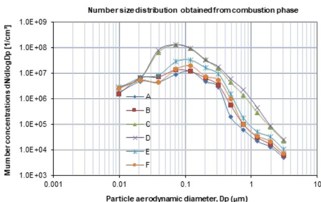
Fig. 11: Particle number size from distributions obtained from the combustion phase of all the experiments
