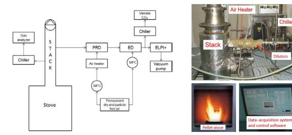
(a) schematic of the experimental setup
