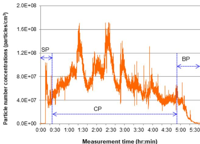
Fig. 8: Time series of particle number concentrations obtained from Experiment C during nominal load output, SP = startup phase, CP = combustion phase, BP = burnout phase
