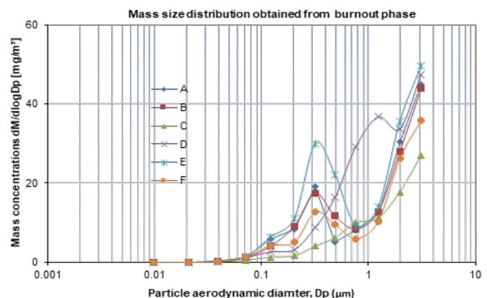
Fig. 7: Particle mass size distributions obtained from the burnout phase of all the experiments
