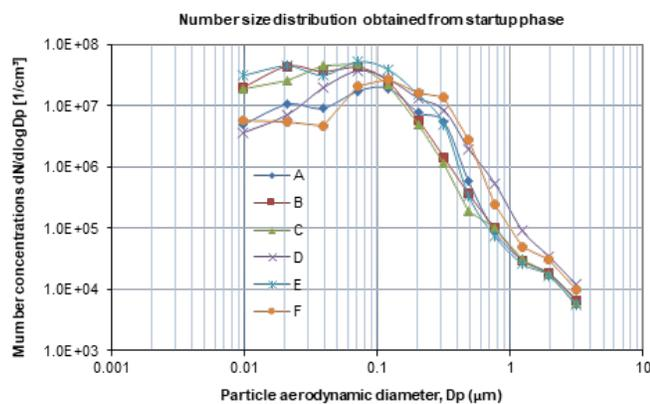
Fig. 10: Particle number size from distributions obtained from the startup phase of all the experiments
