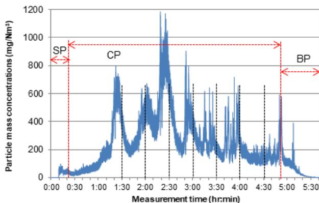
Fig. 2: Time series of particle mass,  $PM_{2.5}$  concentrations obtained from combustion Experiment C, SP = startup phase, CP = combustion phase, BP = burnout phase.
