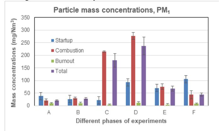
Fig. 3: Comparison of  $PM_1$  concentrations obtained from all the combustion experiments
