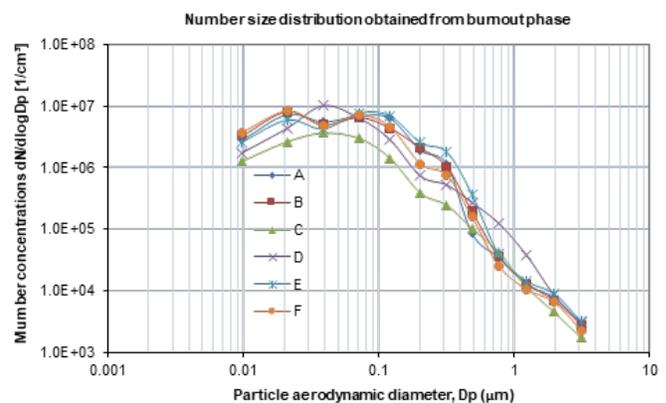
Fig. 12: Particle number size distributions obtained from burnout phase of all the experiments
