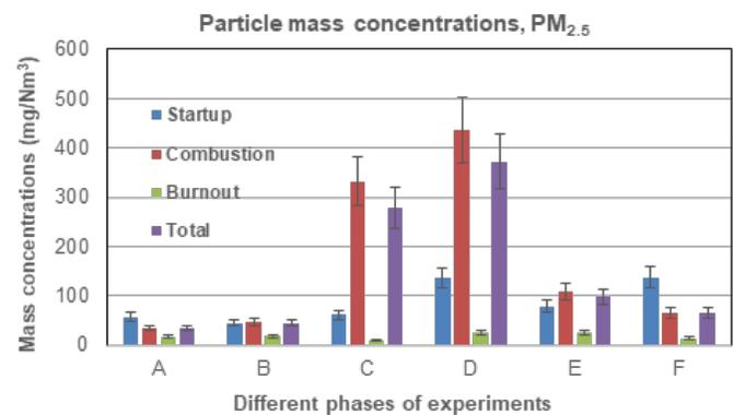
Fig. 4: Comparison of  $PM_{2.5}$  concentrations obtained from all the combustion experiments
