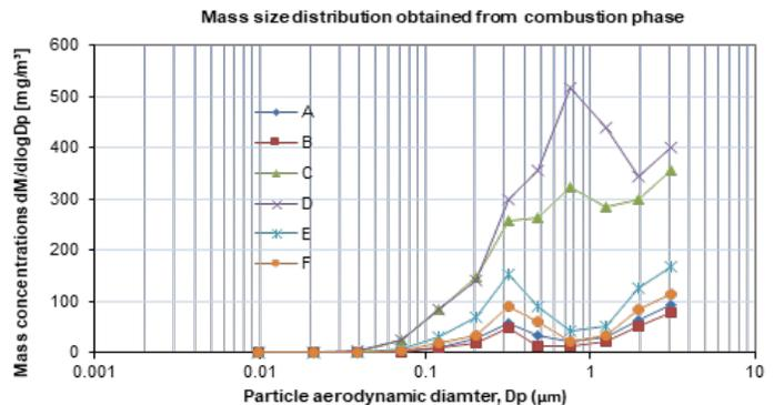
Fig. 6: Particle mass size distributions obtained from the combustion phase of all the experiments
