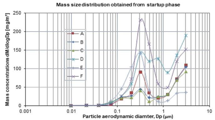
Fig. 5: Particle mass size distributions obtained from the startup phase of all the experiments
