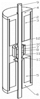
Fig. 6. Braille Display element.
