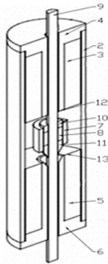
Fig. 6. Braille Display element.
