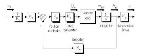
Fig.1 a simplified block diagram for a NC feed drive.
