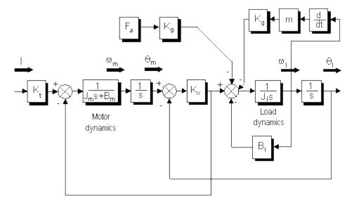
Fig.2 A detailed diagram of the behavior of the mechanical system.
