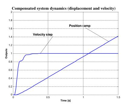
Fig.8 Dynamic response of compensated system- displacement and velocity.
