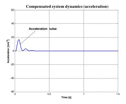
Fig.9 Dynamic response of the compensated system – acceleration.
