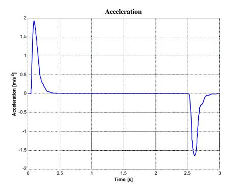
Fig.12 The result of simulation in positioning regime – acceleration.
