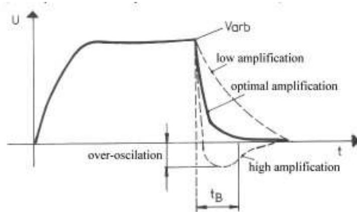
Fig.5 The way of exponential deceleration of a slide.
