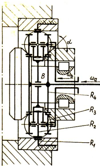
Fig.4 Scheme of a planetary mechanism used for the rolling operation.
