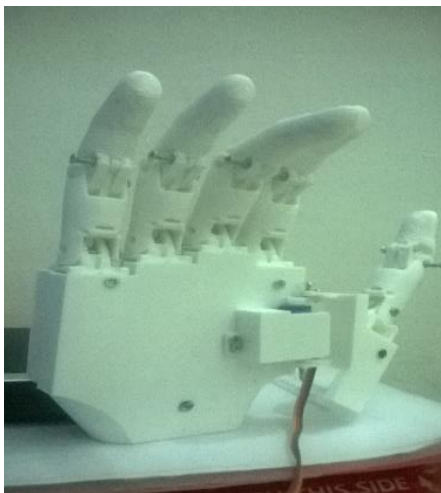
Fig. 6. Prototype of the hand during construction phase
