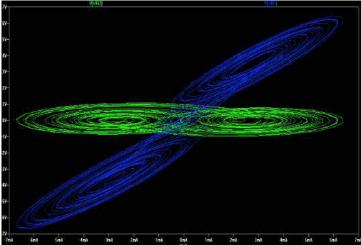
Fig. 6 The Double-Scroll attractor pattern obtained by plotting  $V_2$  (in green) and  $V_l$  (in blue) with respect to  $I_L$
