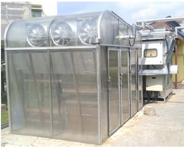
Fig. 5 Drying chamber and dryer system
