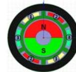
Fig. 3 Three coils (1, 2 and 3) and a permanent magnet in the cross-section of a BLDC motor
