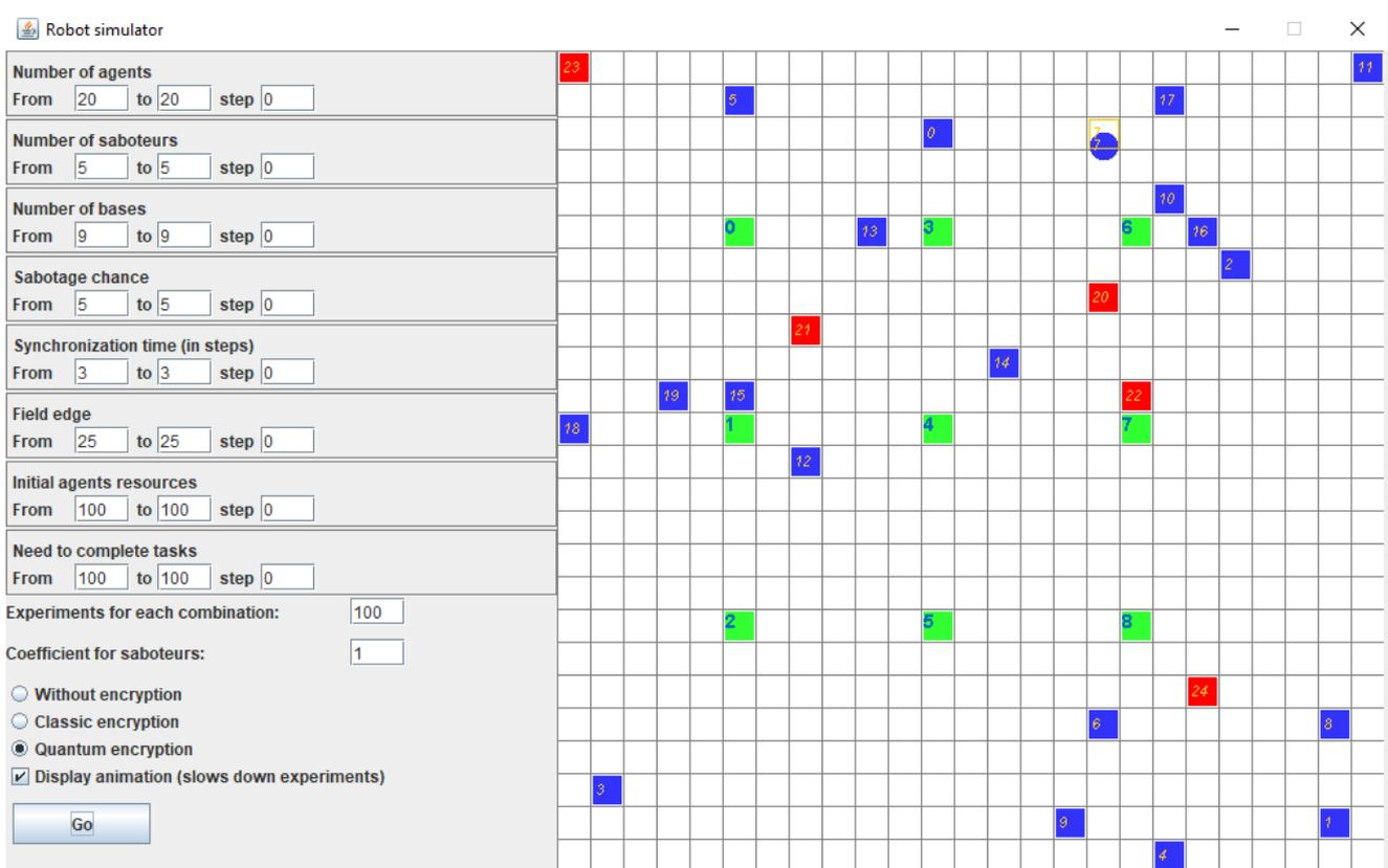
Fig. 6. Graphical interface of the MARS functioning software simulator. Blue color indicates allied agents, red - saboteurs, green – bases. The parameters of the experiment are set on the left side of the interface.
