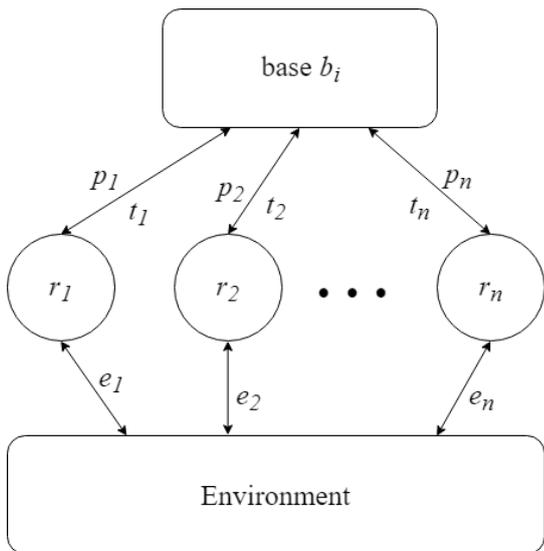
Fig. 4. Diagram of the low-level interaction between robots and bases
