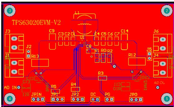
Fig.5 DC-DC converter circuit PCB component layout
