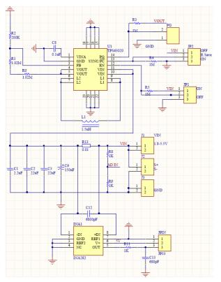
Fig.4 DC-DC conversion circuit schematic
