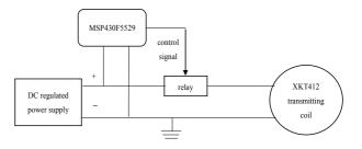
Fig.1 Wireless charging transmitter system block diagram
