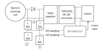
Fig.2 Wireless charging receiver system block diagram
