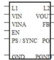
Fig.3 TPS63020 pin diagram
