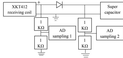
Fig.6 Sampling schematic
