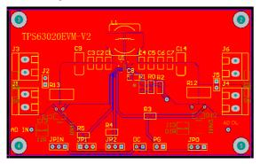
Fig.5 DC-DC converter circuit PCB component layout
