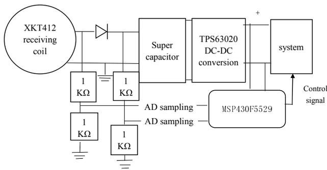
Fig.2 Wireless charging receiver system block diagram
