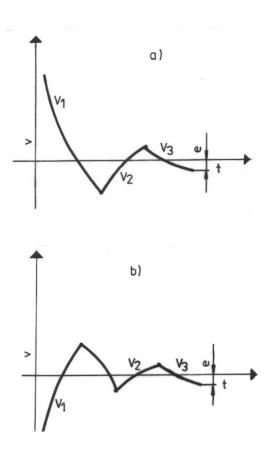
Fig. 1 a) Response with over-oscillation; b) Response with over-oscillation from the same direction, for backlash take-over.
