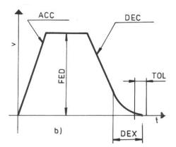
Fig.8 a) Poisoning feed linkages where a dead stroke exists; b) Contouring feed linkages with parameters adjusted
