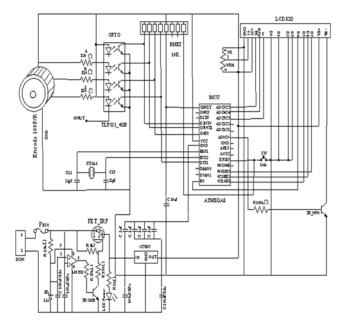
Fig. 2. The contact tachometer circuit
