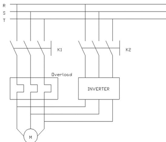
Fig. 1. Compressor connection before and after installation VSD.
