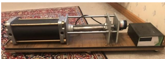
Figure 2. computer-controlled, step motor driven air pump used to perform different waveforms.
