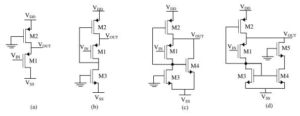
Fig 2 Voltage buffer: (a) common-drain, (b) Flipped voltage follower (c) Folded flipped voltage follower, (d) Modified folded flipped voltage follower
