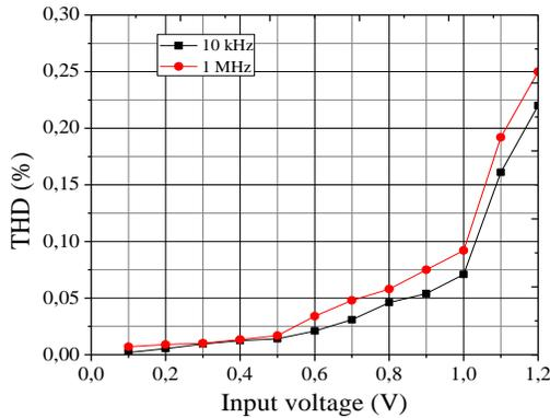
Fig. 10 THD of voltage follower with 10 kHz and 1 MHz.
