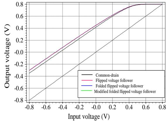
Fig. 3 DC voltage transfer characteristics
