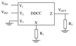
Fig. 11 Voltage mode instrumentation amplifier circuit (VMIA)
