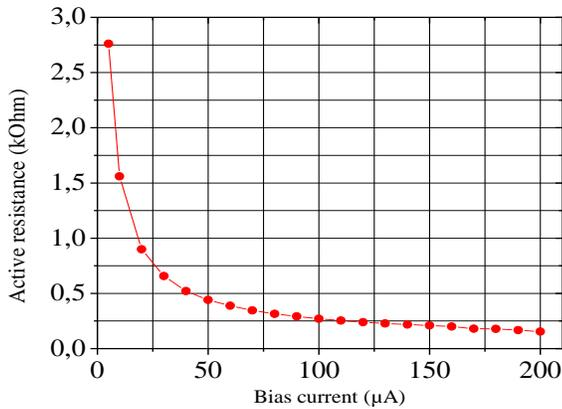
Fig 14. Variation of active resistor and center frequency values according to bias current  $I_0$
