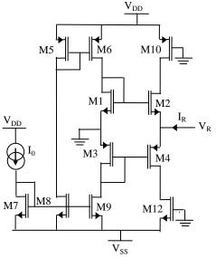
Fig 13. Active resistance controlled by bias current  $I_0$
