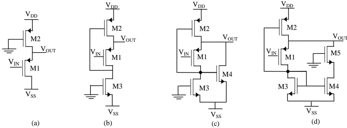
Fig 2 Voltage buffer: (a) common-drain, (b) Flipped voltage follower (c) Folded flipped voltage follower, (d) Modified folded flipped voltage follower
