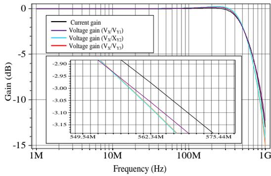
Fig. 8 Frequency responses of current and voltage gains
