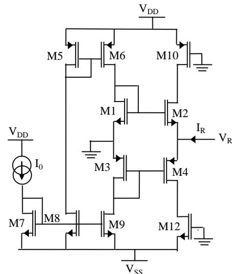
Fig 13. Active resistance controlled by bias current  $I_0$
