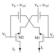
Fig. 1 Schematic diagram of differential pair biased by adaptive biasing circuit
