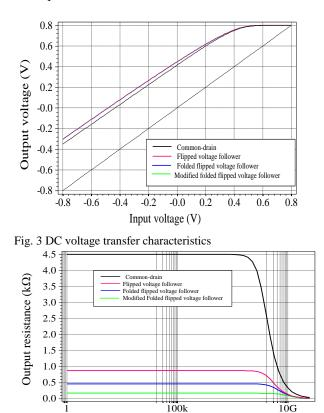
Fig 4 Variation of output impedances according to frequency
