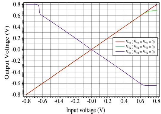
Fig. 6 DC transfer characteristic for voltage transfer
