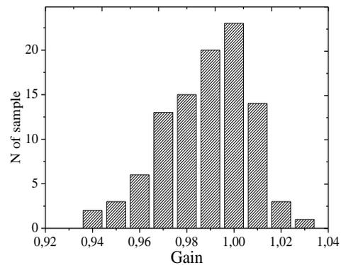
Fig 18. Statistical results of Monte-Carlo analysis for VMIA with 10% deviation bias current  $I_0$
