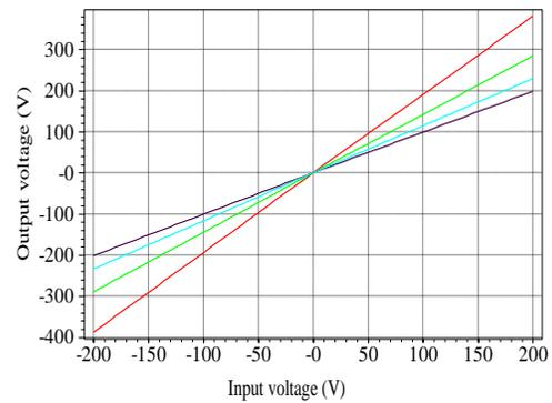
Fig 16. DC transfer characteristics of VMIA
