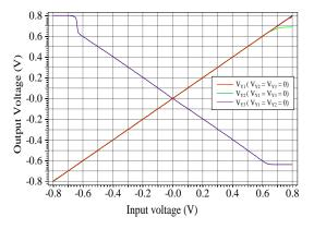
Fig. 6 DC transfer characteristic for voltage transfer
