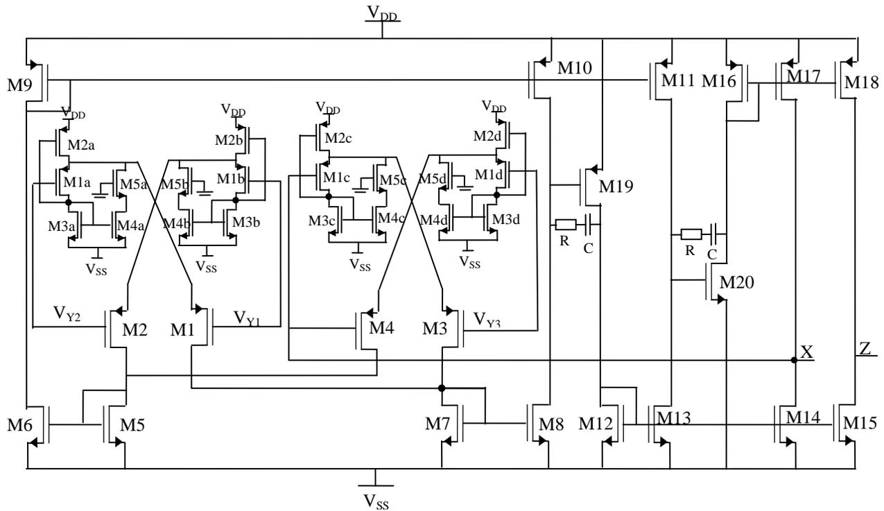
Fig 5. Proposed differential difference current conveyor circuit (DDCC)
