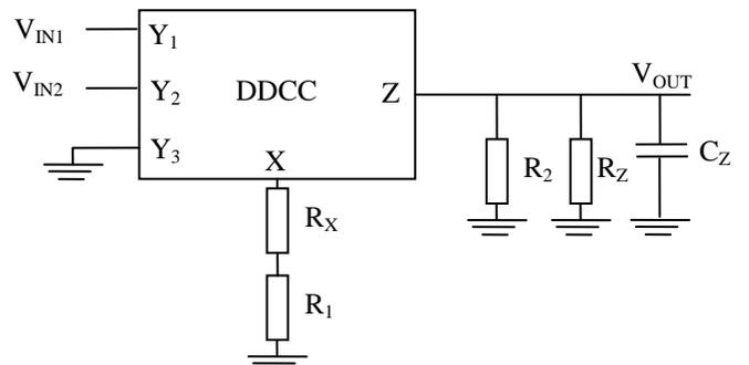
Fig. 12 Instrumentation amplifier circuit considering the present of parasitic elements
