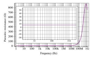
Fig. 9. Frequency response of parasitic impedance Z<sub>X</sub>
