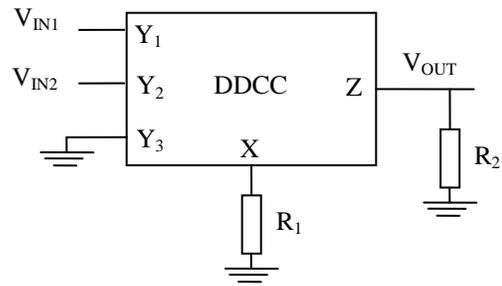
Fig. 11 Voltage mode instrumentation amplifier circuit (VMIA)
