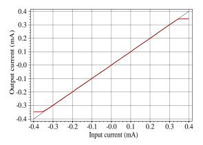
Fig. 7 DC transfer characteristic for current transfer
