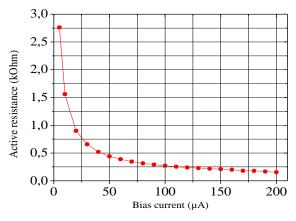
Fig 14. Variation of active resistor and center frequency values according by bias current  ${\rm I}_0$
