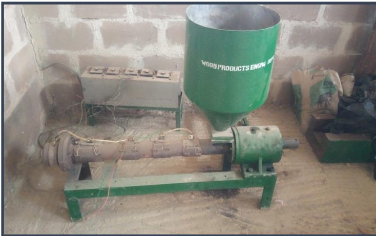
Fig. 5: Locally fabricated Single Screw Extruder Machine
