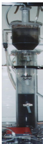
Fig. 1. Laboratory-scale UASB reactor used in this work.
