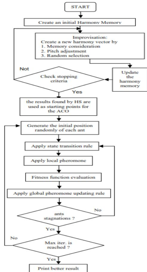
Fig. 1. Flow chart for EPD using HSA-ACO.
