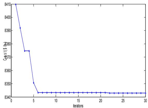
Fig. 2. Convergence characteristic for fuel cost minimization (3-unit system, demand 850 MW).
