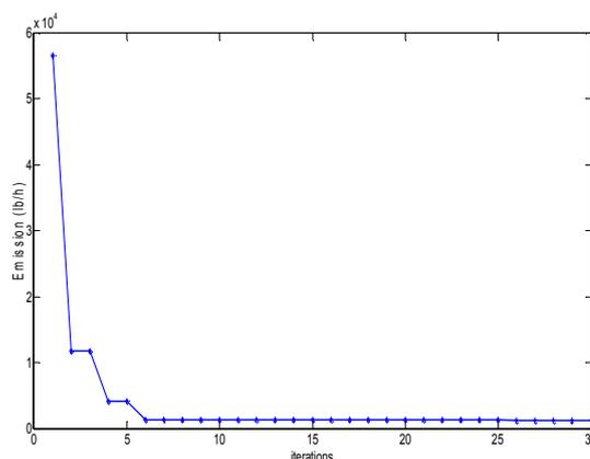
Fig. 6. Convergence of emission for 6-unit test system.
