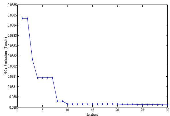
Fig. 4. Convergence characteristic for NO<sub>x</sub> emission minimization (3-unit system, demand 850 MW).
