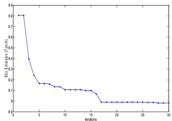
Fig. 3. Convergence characteristic for SO<sub>2</sub> emission minimization (3-unit system, demand 850 MW).
