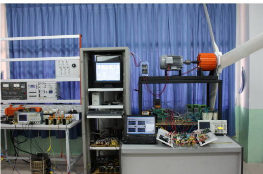
Fig 3: Developed prototype wind system including monitoring system
