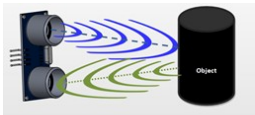
Fig. 4. Function of the Ultrasonic Sensor.
