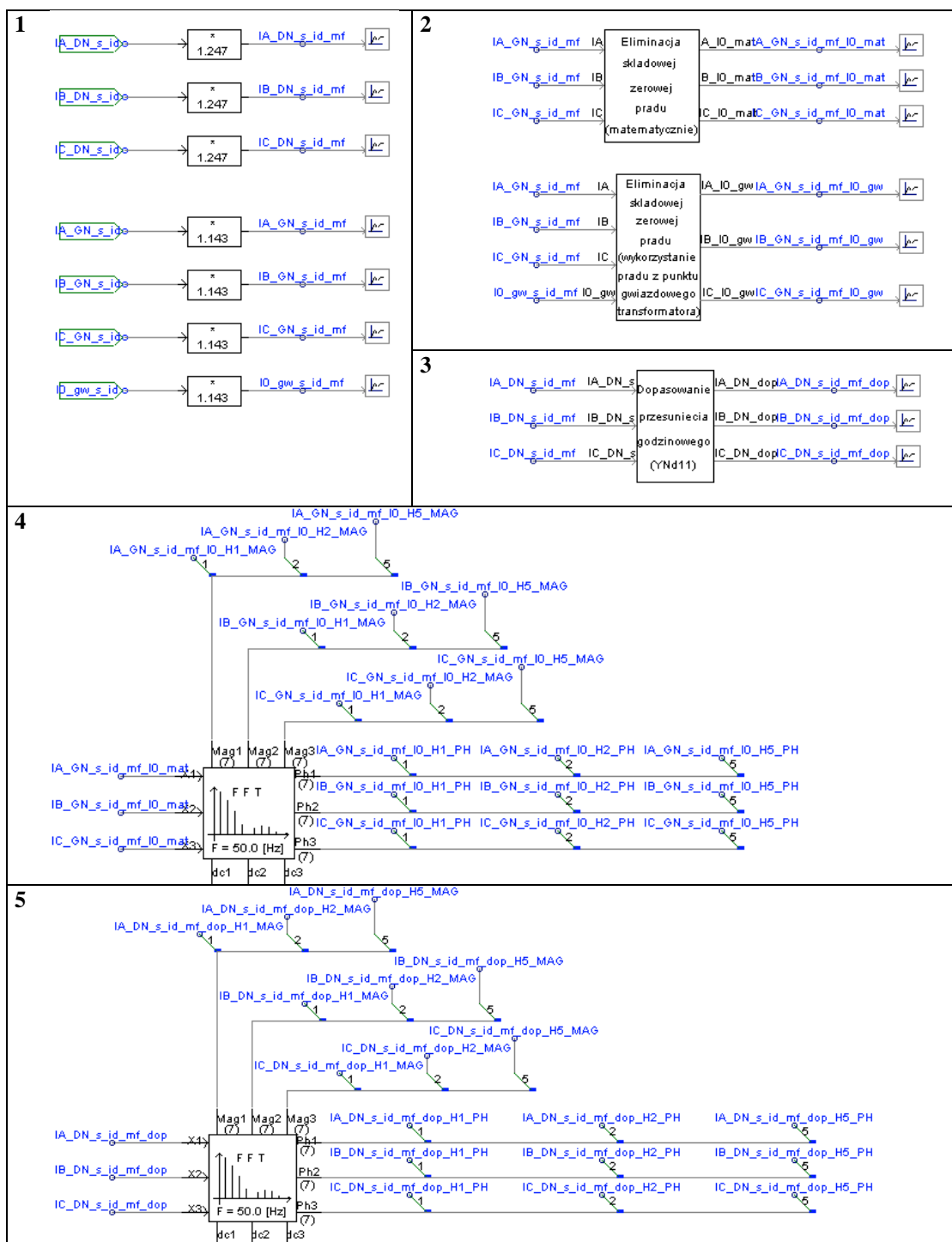
Fig. 3a. Implementation in PSCAD/EMTDC software the modelled relay for protecting the 110 kV/15 kV transformer with YNd11 vector group - scheme 3 (Part 1)
